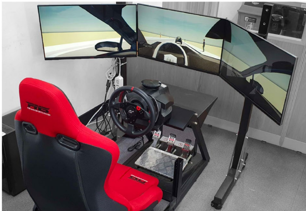
Fig. 1 L2 automated driving simulator. The lower left section shows the movable seat and desktop computer. The center shows the Thrustmaster’s T500RS racing-wheel set and the Jabra Speak 510 speakerphone. The upper right section shows the experimental scenario screen.
